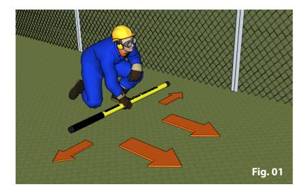
To locate, position your magnetic locator horizontally above the ground (Fig. 01), with its long axis perpendicular to the fence. With this, you make sure that the middle sensor is kept away from the fence.
