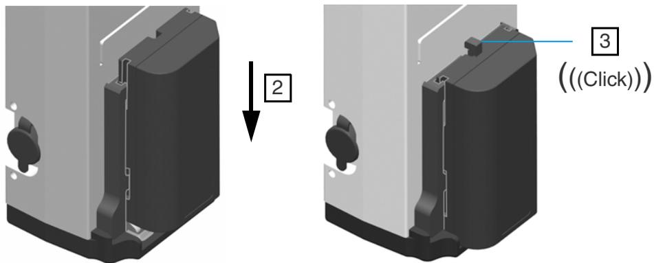
Figure 5.21 Fitting battery to external radio
