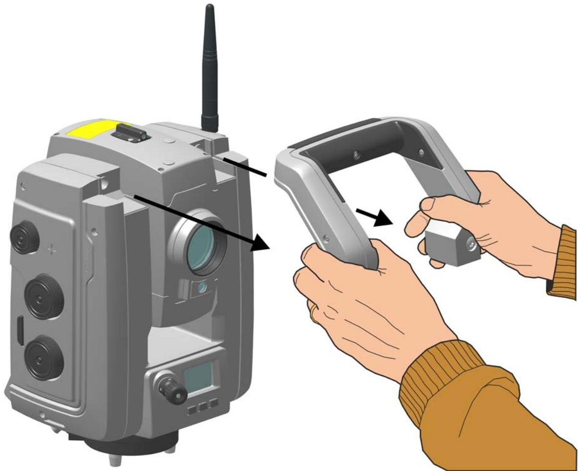
Figure 2.14 Detaching the instrument handle
