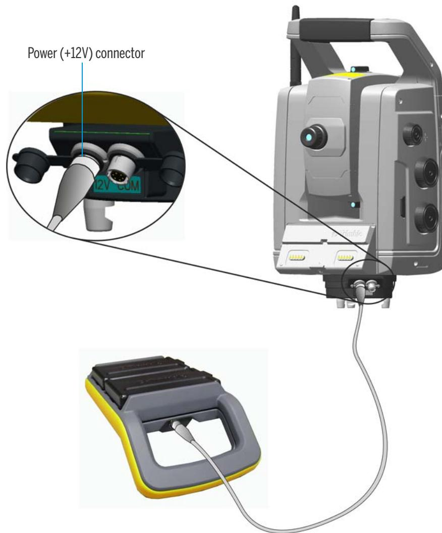
Figure 5.2 Connecting the Multi battery Adapter
