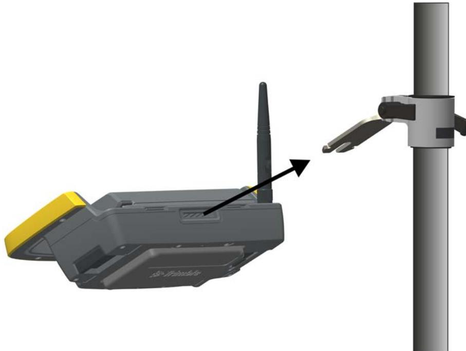
Figure 5.17 Attaching the Trimble Robotic Holder to the standard rod adapter
