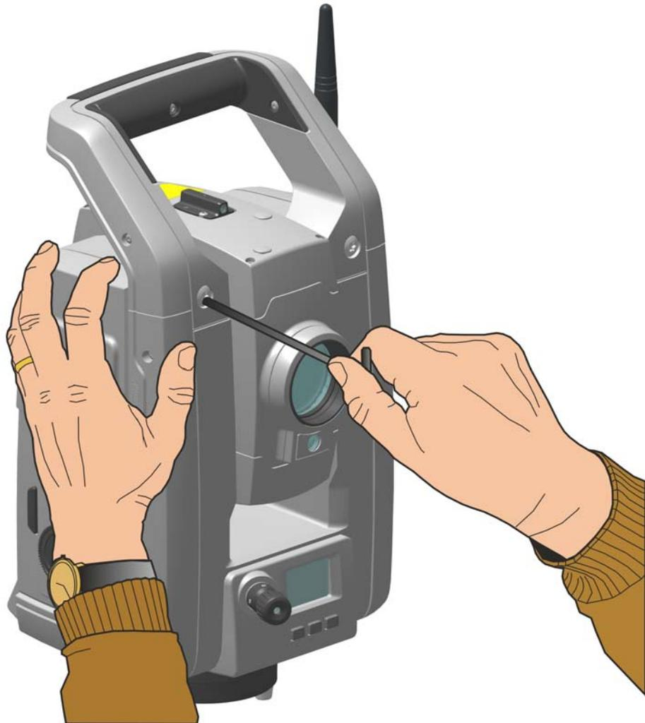
Figure 2.13 Removing the instrument handle
