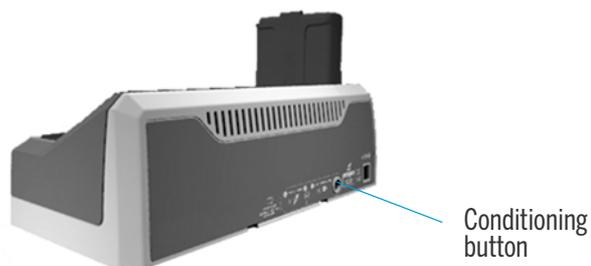
Figure 2.4 Battery charger conditioning button
