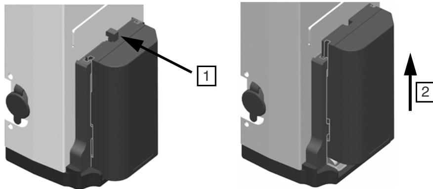
Figure 5.22 Removing battery from external radio
