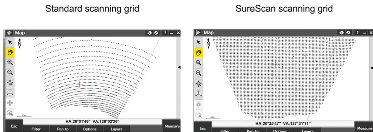
Figure 4.9 Standard scanning grid compared to SureScan scanning grid.
