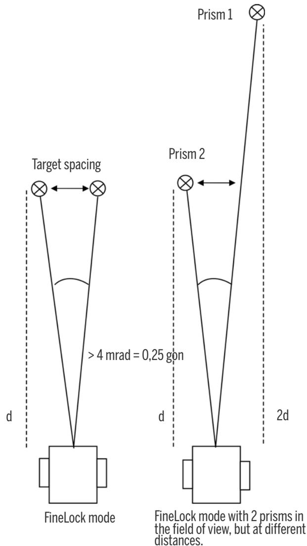
Figure 4.6 Measuring in FineLock mode
