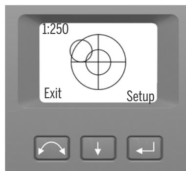
Figure 2.11 Electronic leveling screen on the face 2 display
