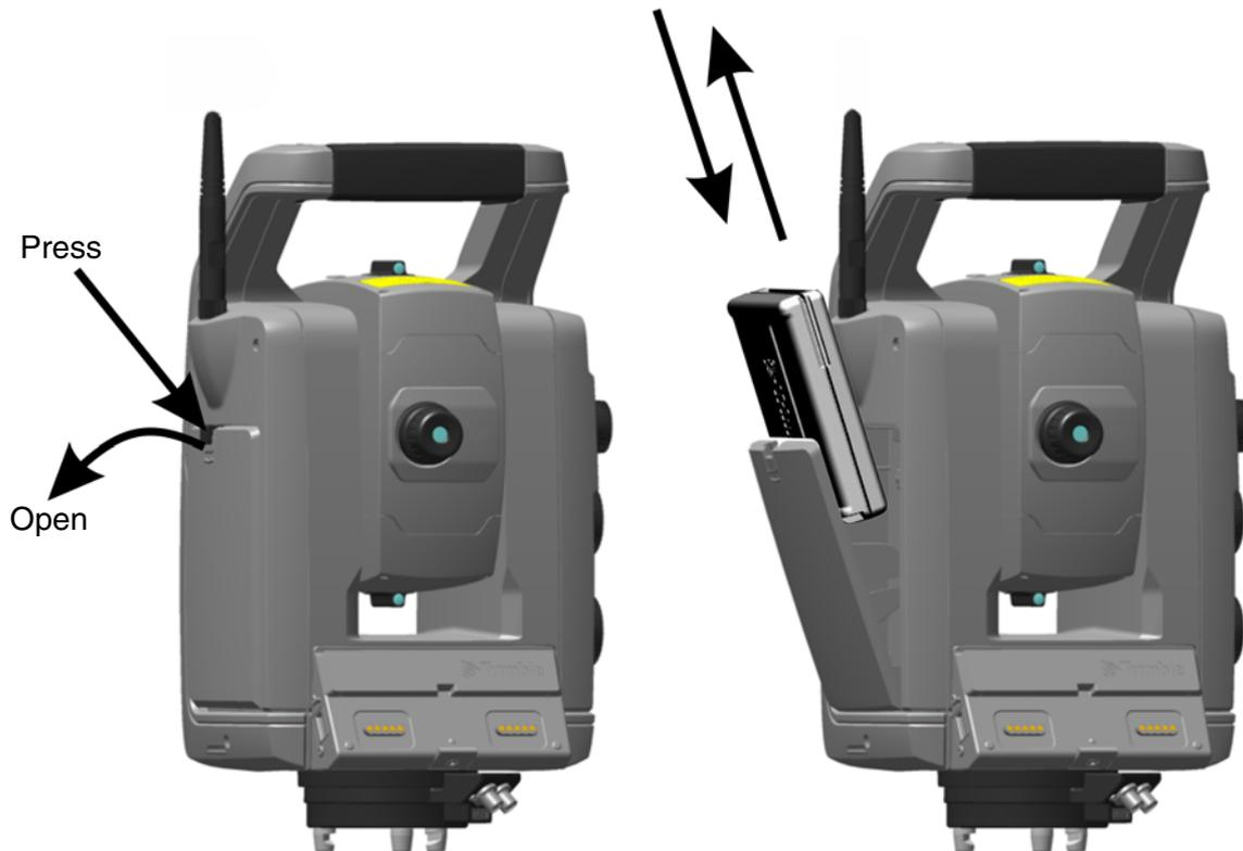
Figure 2.7 Inserting and/or removing the internal battery
