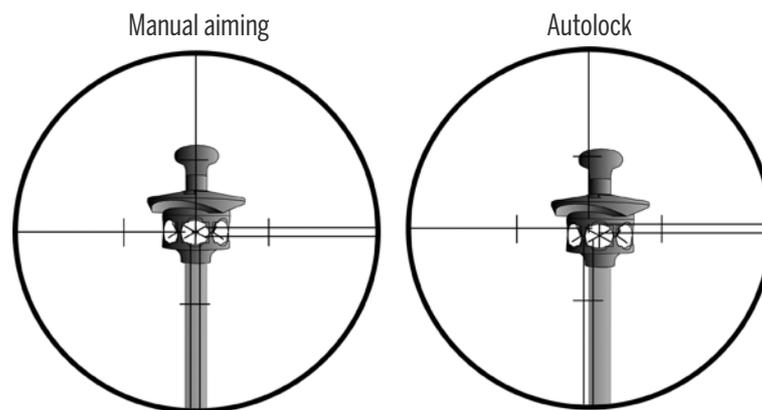
Figure 4.7 Difference between aiming manually and Autolock
