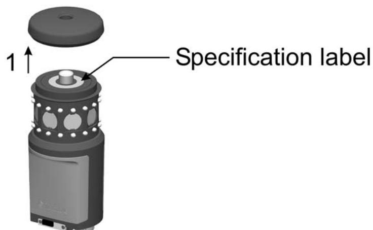
Figure 5.11 Location of Trimble MultiTrack Target specification label
