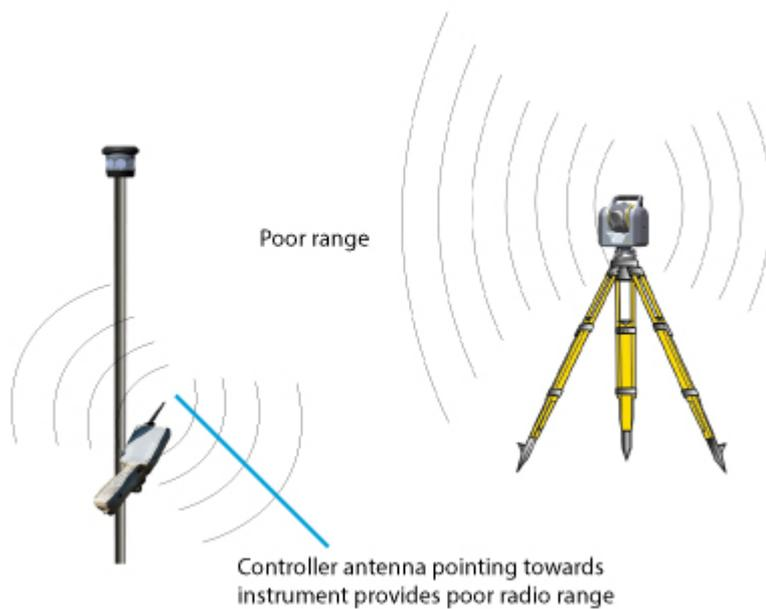
**Poor radio range with controller antenna not in the same vertical position as the instrument antenna**
