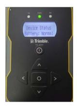
The first screen you will see is the Device Status Battery Normal screen. Press the right arrow key to view the following settings for the Trimble R8 and R10 receivers. Please note that after every change the center circle button must be pressed. Once the center button is pressed, a star will show up on the left side of the screen denoting that the setting has been saved
