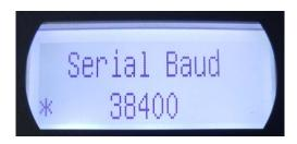
These settings will get you up and running with the R8 and R10 receivers. Duplicate these settings in the internal radios of the rovers. The frequency, radio link rate, and serial baud rate in the rover must match exactly to receive the signal from the base.
