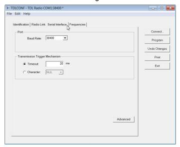
The Serial Interface screen lets you set the baud rate at which your radio will communicate with external devices such as computers, GNSS receivers or monitoring equipment. In general, the higher the baud rate the better, but whatever value you chose, you must configure the external device with the same rate.
