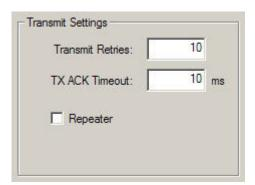
The Transmit Retries feature only works when the addressing feature is enabled. When addressing is enabled, the receiving radio will send an
