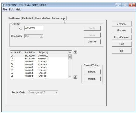
The Frequencies screen displays the channel table created for you by your dealer. This channel table consists of one or more channels with RX and TX frequencies, a channel bandwidth used for all channels and a region code.
