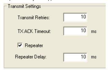
**Note** – Only the PCC EOT protocol supports transmit retries. So when you select any other protocol in the **Protocol** selection field (see above), the **Transmit Settings** section of the **Radio Link** screen does not display the **Transmit Retries** or **TX ACK Timeout** check boxes.
