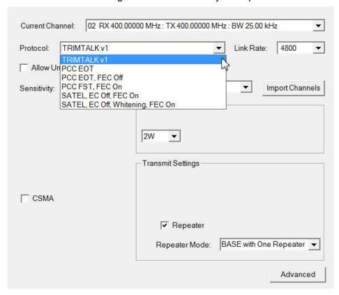
TRIMTALK v1 is an improved version of all of the older Trimble protocols, such as TRIMTALK 450S, TRIMTALK II/IIe, TRIMMARK 3, etc. It is backward compatible with all of these older versions.
