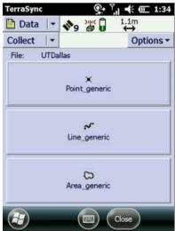
\*\*\*If the unit does not automatically connect in Step 3, navigate to the "Setup" window and ensure you are connected to the GNSS receiver by tapping the GNSS in the upper right-hand corner\*\*
