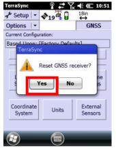
6. Once the receiver resets, please allow 10-15 minutes for the unit to download an updated Almanac. The unit should begin to track satellites within that window of time. Ensure the unit has a clear view of the sky to initiate satellite tracking.
